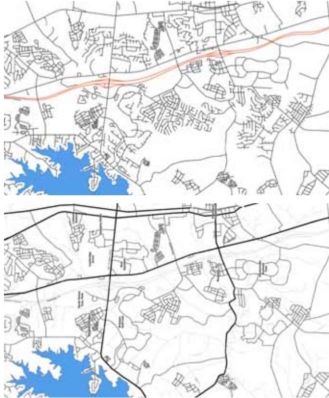
EFFECTIVE STREET NETWORK (LEFT) AND THE EXISTING STREET PATTERN. These diagrams show all the effectiveness of a network of streets that contribute to the regional transportation network. The first diagram removes all streets that are cul-de-sac, and streets that do not connect to more than one roadway. Both interchanges show a very sparse network of streets resulting in a few connected links conveying both the regional and local traffic.
