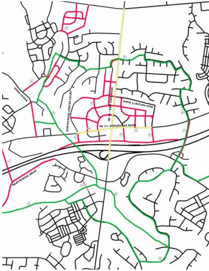
PROPOSED STREET FRAMEWORK New streets and a modified ramp system will create a more connected community and will help transition the area from a suburban commercial center to a mixed-use town center.
